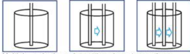
Multiple aspiration point settings (one, two or three positions) to optimize liquid aspiration from different plate types
